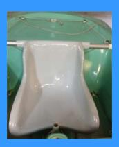
The Universal Bucket seat is a fiberglass seat which can be retro-fitted to any 2.3 or 303 wide.
